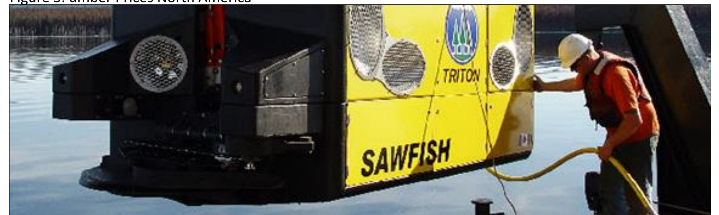
Figure 4. Remote Operated Vehicle (ROV) Sawfish From Triton Company
