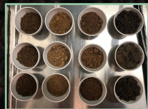
Preparation of samples for organic matter content determination via loss on ignition
